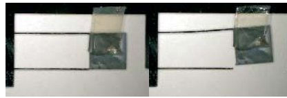
Figure 5: Deformation of a silicon structure due to the shrinking of FULCEa
