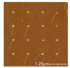
desirable. To this end, E. Delamarche and co-workers demonstrate single virus arrays by using direct printing of unmodified anti-M13 bacteriophage antibodies onto silicon with nanometer resolution, widely variable feature pitch, and flow alignment of the viruses. Such functional, addressable arrays may find interesting applications, including microarray technology and bottom-up nanoassemblies. /sos
