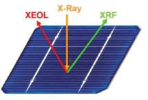
information yield. They show that it is possible to perform X-ray-excited optical luminescence (XEOL) on crystalline silicon despite the fact that its indirect bandgap causes low luminescence efficiency. In order to establish this new approach, XEOL data from two samples with high and low minority carrier lifetime is compared to conventional luminescence and X-ray fluorescence. /sb
