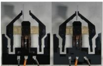
that it is suitable for slow, sensitive positioning and gripping movements. On applying electrical power, the nematic-to-isotropic transition induces changes in the LCE film length, causing strains of up to 150% and the capacity to move up to 400 times its own mass! /lb
