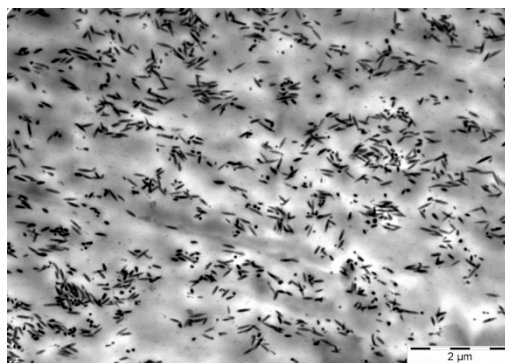
Figure S1 TEM micrographs of the liquid-crystalline elastomer nanocomposite: different regions in the sample all proof the good dispersion with occasional small aggregates of several particles.
