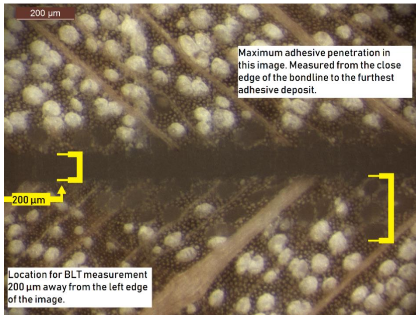
Fig. SI-2: Visualisation of the location for measuring the bond line thickness (BLT) and the maximum adhesive void penetration (MAP) on the example of unprimed beech wood bonded with 1c-PUR.
