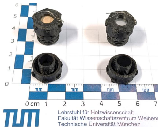
Fig. SI-1: (Left) Schematic drawing of three-piece cups with the wood specimen placed between the upper and middle part, as well as the bottom part filled with water. (Right) Measurement cups with the wood specimen (above, left) and the aluminum reference (above, right) fixed between the upper and middle piece and the bottom part with the water bin in front (below).
